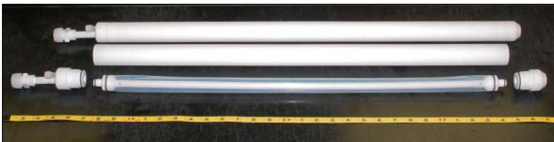
Figure 9. Example of a Teflon® constructed bladder pump, complete (top) and exploded version illustrating internal Teflon® bladder (Photograph by J. Schoenleber)
