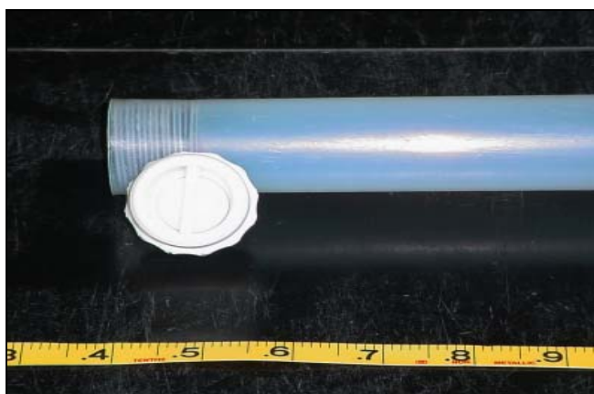
Figure 7. Teflon® constructed bailer with Teflon® ball check valve (Photograph by J. Schoenleber)
