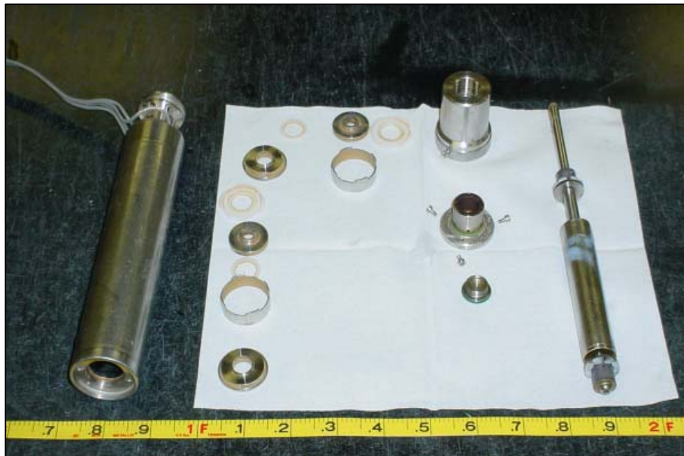
Figure 11. Disassembled Grundfos® Pump being prepared for decontamination (Photograph by J. Schoenleber)
